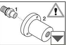
Clean spindle end and bore where rotor will be installed. Slightly lubricate spindle end for stub rotors.
