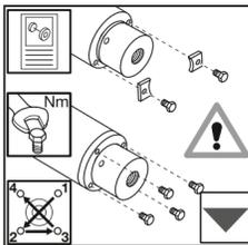
Before connecting hoses, on unions with axial supply port carefully push the floating seal with a suitable object forward again until it touches the rotor seal. For **all** models pertains: Apply repeated air pulses > 6bar until no air leakage is observed from the union.
