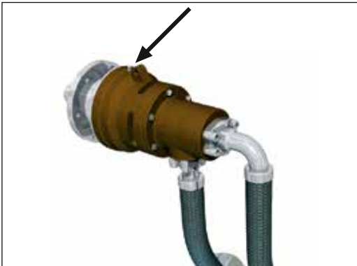
Fig. 8: Attach grease gun for relubrication
