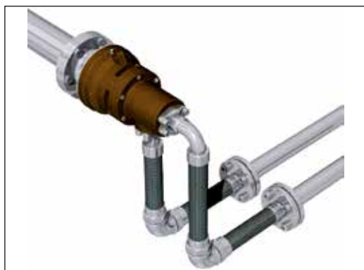
Fig. 5: Hoses bent by 90°
