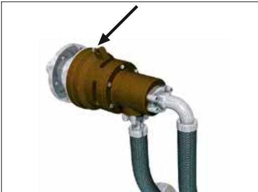
Fig. 8: Attach grease gun for relubrication
