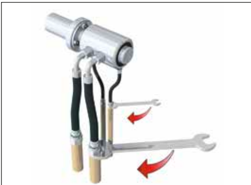
Fig. 4: Connect hoses with 90° elbows
