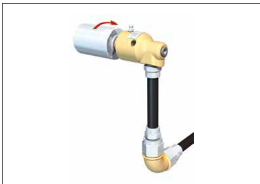
Fig. 7: Hoses bent by 90°
