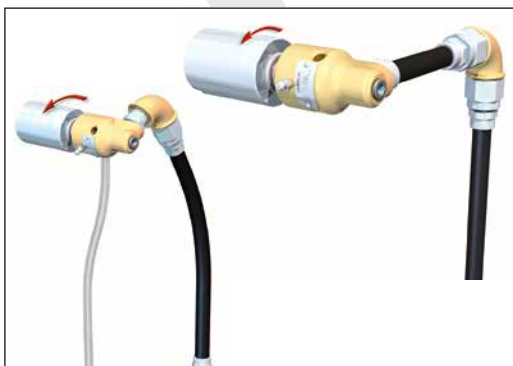
Fig. 6: Connect hoses horizontally
