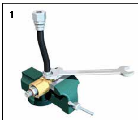
Mount housing in a bench vise and install hose.
