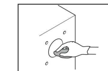
Ensure roll bore is clean and free of debris and burrs.
