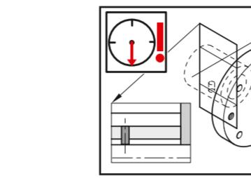
When inserting the rotating union make sure that the pin fits into the keyway of the rotor. Flange must fit flush against bore.
