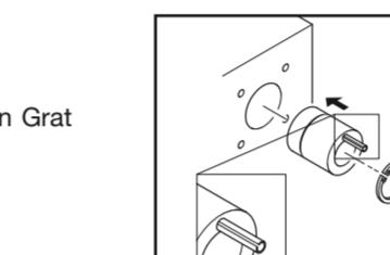
Insert bushing into the roll with axial driving pin outside. Secure with snap-ring (if supplied).
