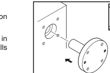
Secure retaining plate/flange by tightening the screws in a star pattern.
