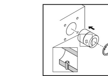
Insert bushing into the roll according to **DEUBLIN**'s specification (technical drawing), secure with snap-ring (if supplied).
