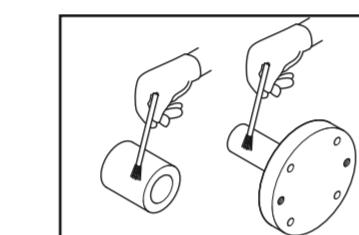
Lubricate the union housing and bushing before inserting the housing into roll bore.
