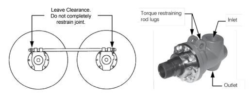
Torque restraining rods may be installed either horizontally, when rolls are alongside of each other, or vertically, when rolls are in stacks above each other.
