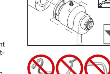
**Option:** Connect flange rotor. Secure flange by tightening bolts in a star pattern.
