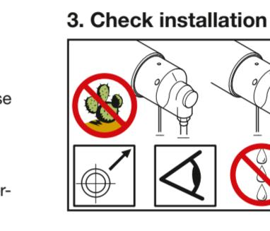
Check the union for leakage.
