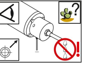
Check the union for leakage at the supply and drain fittings.
