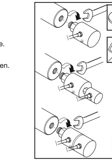
Attach the **DEUBLIN** Rotating Union onto the shaft with sealant, PTFE tape or gasket.
