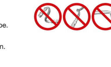
Arrange and connect the hoses without any strains, torsional stress or sharp bends.
