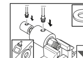
Attach appropriate, flexible hoses with sealant or PTFE tape.
