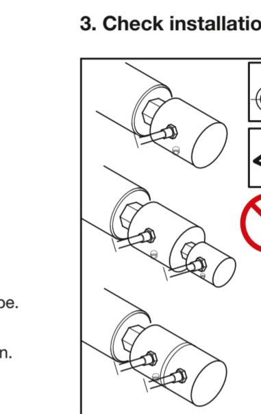
Check the union for leakage.
