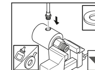
Attach appropriate, flexible hose with sealant or PTFE tape.
