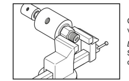
Chuck the **DEUBLIN** Rotating Union ONLY at the rotor onto a vise as shown. Attention: Don't damage aluminium housing.
