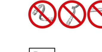
Arrange and connect the hoses without any strains, torsional stress or sharp bends.
