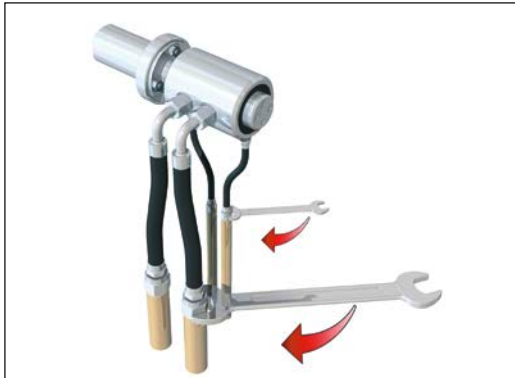
Fig. 4: Connect hoses with 90° elbows
