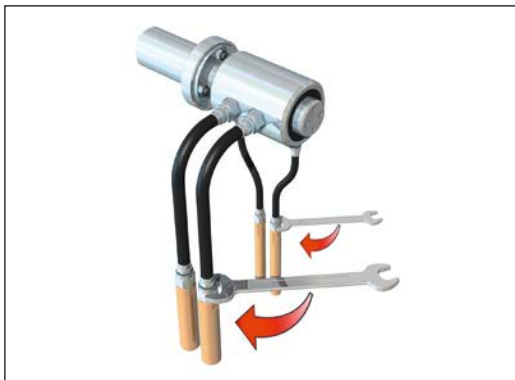
Fig. 5: Connect hoses with straight connections
