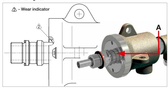
Fig. 10: Wear indicator on the rotor
