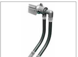
If you want to connect the rotating unions to a machine then you must make the connection with flexible hoses. Flexible hoses prevent any side loads occurring on the rotating union's bearing during operation.
