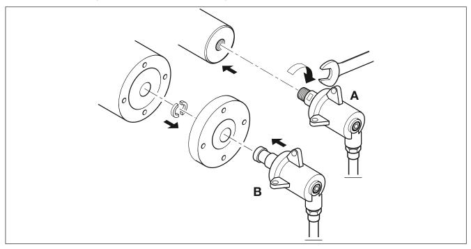
Fig. 4: Options for the installation on the machine shaft
