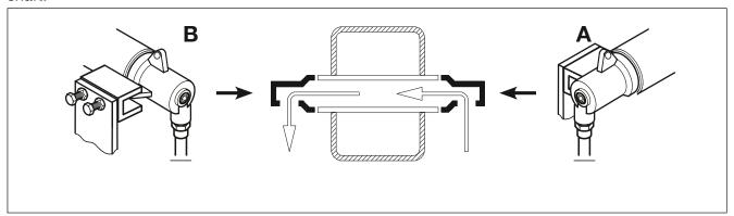
Fig. 1: Schematic diagram single passage version (Mono – externally mounted)
