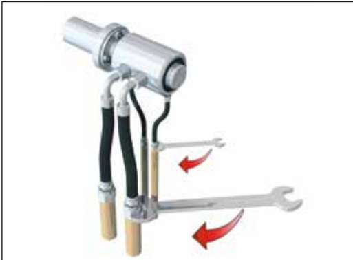
Fig. 4: Connect hoses with 90° elbows
