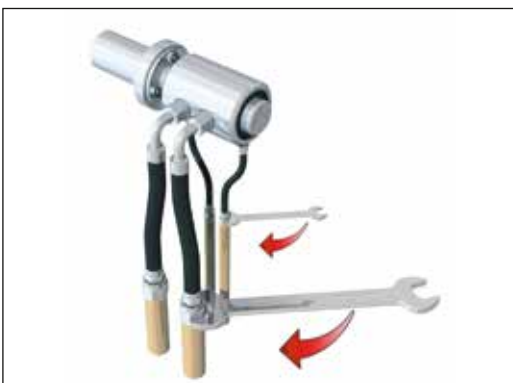
Fig. 6: Connect hoses with 90° elbows
