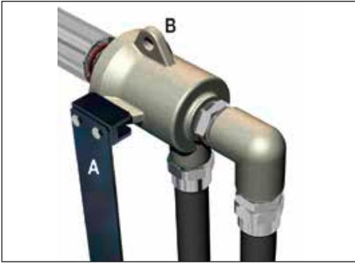
The rotating union housing must be secured against rotation during operation using an anti-rotation element **(A)**. For this the rotating unions are fitted with torque supports **(B)** on the housing. The anti-rotation devices can be attached to these torque supports but must not prevent axial movement.
