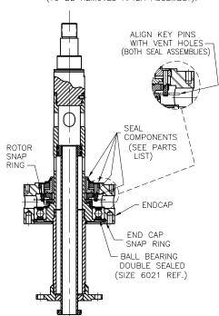
ENDCAP-SNAP RING SEAL COMPONENTS (SEE PARTS LIST) HOUSING (WITH BEARING **ENDCAP** INTACT) BOLTS BOLTS 3/8-24 X 1 1/8 - END CAP REMOVE (4) KEY PINS (2) EACH END-
