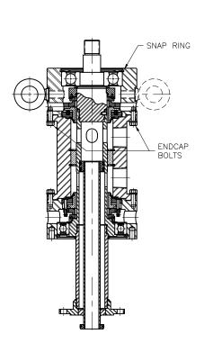
2. SUPPORT ENDCAP BY EYEBOLTS AND PRESS ROTOR AND REMAINING PARTS OUT OF ENDCAP.
