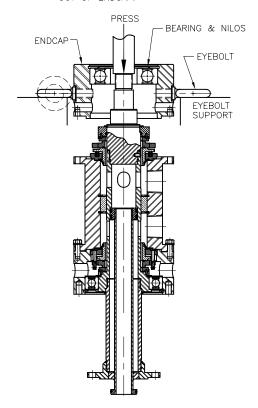
3. REMOVE ROTOR SNAP RING AND SEAL COMPONENTS AS SHOWN.
