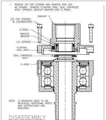
2. INSPECT ENDCAP BORE FOR WEAR OR PITTING. BORE SHOULD BE SMOOTH AND TO SIZE SHOWN.
