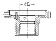
CAP ROTOR AND PUT MASKING TAPE OVER ALL BUT ONE VENT HOLE. APPLY AIR PRESSURE. BRUSH SOAP WATER SOLUTION OR BUBBLE SOAP TO VENT HOLE. ROTATE UNION BY HAND; IF NO BUBBLE RISES, UNION IS O.K.
