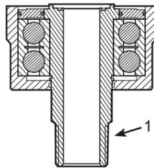
Place Rotor (1) on end while protecting threads from damage. Lubricate O-ring (2) with Grease (TS08). Assemble O-ring (2) and Rotor Seal Sub-assembly (3) onto the Rotor as shown and apply three drops of Lubrication oil (TS07) to the Rotor seal face.
