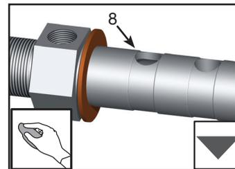
The surface finish of the rotor (8) OD must meet Ra 0.4  $\mu\text{m}$ . If not, it should be replaced. Clean housing (7) and rotor (8) thoroughly before reuse.
