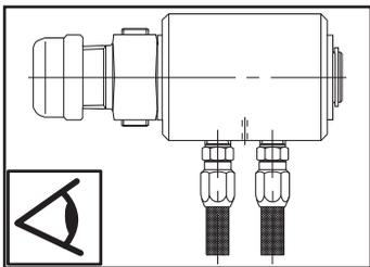
Put soap solution over drain hole while rotating rotor by hand. If no bubbles rise up, union is good for installation.
