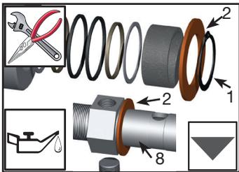
Apply light oil on the outside of the rotor. Install thrust washer(s) (2) to rotor (8). Insert rotor into housing assembly with arbor press. Install thrust washer (2) and snap ring (1).
