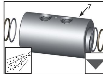
The housing (7) may be grit-blasted with glass bead or aluminum oxide to remove dirt and debris. **Sand-blasting is NOT recommended.**
