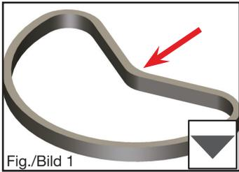
**Hint:** slightly bend (no twist) slipper seals (5) as shown in figure 1 before placing them into the housing grooves.
