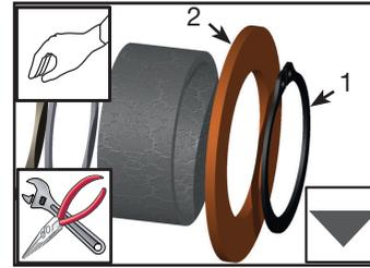
Remove snap ring (1) and thrust washer(s) (2). Press out rotor (8) with arbor press.
