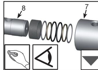
Clean housing (7) and rotor (8) thoroughly. Visually inspect for any surface defects inside the housing or on the outside of the rotor.
