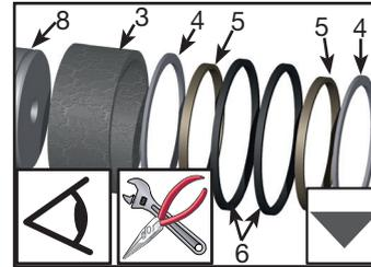
Inspect for surface defects on composite bearings (3). If they have any, union should be sent back to *DEUBLIN* for rebuild or should be replaced by a new unit. Remove and discard slipper seals (5), square cut rings (6), and backup washers (4) by piercing with a sharp pointed tool.
