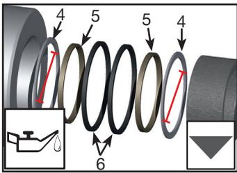
Install backup washers (4), and square cut rings (6) to housing. Apply light oil on square cut rings (6). Check that square cut rings (6) are not twisted. Place slipper seals (5) over square cut rings (6).
