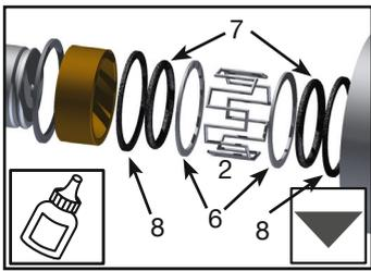
Apply silicone-based grease to all o-rings (7). Install backup washers (8), O-rings (7), seal guide (6), and to serpentine spring (2) housing (1).
