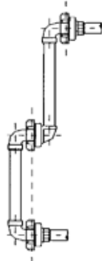
Correct 2 joints in line
