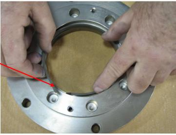
**Step 27:** Grease outside of new C-ring. Insert C-ring into outer counterbore of Flange.
