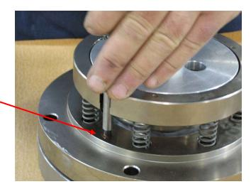
**Step 35:** Lift assembly off of fixture and look at C-ring from bottom. Ensure Slydring is seated properly and not hung up on Flange.
