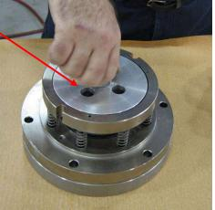
**Step 33:** Place anti-seize compound on 2 screws that hold Carrier to Flange.
