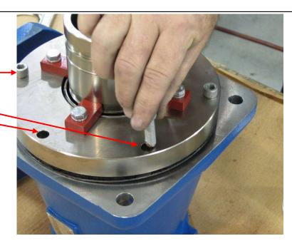
**Step 71:** Tighten down and torque 6 bolts to 35 ft-lbs.
