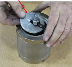
**Step 8:** Tighten nut down to release pressure from Retaining Ring.
