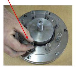
**Step 30:** Grease the smaller outer diameter of the Carrier.
