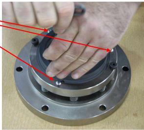
Step 20: Remove O-ring from Carrier.
