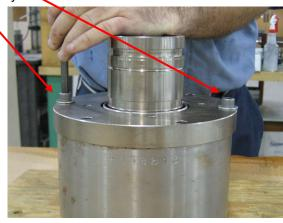
**Step 51:** Insert 4 Red Rotor Tabs onto Flange and slide end of Tabs into groove in Rotor.
