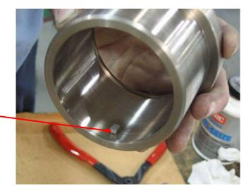
**Step 55:** Insert Carbon Bearing into Retaining Flange. Slot in Carbon Bearing must be aligned with Pin for Carbon Bearing to fully seat.
