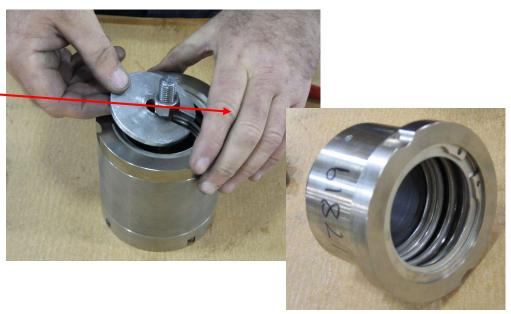
**Step 63:** Grease O-ring and slide over outer diameter of Retaining Flange until O-ring is butted up against shoulder.
