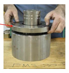
**Step 19:** Remove the 3 screws to remove the front Carbon Seal.
