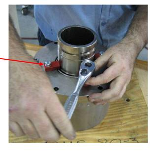
**Step 53:** Remove 2 bolts from Flange and remove Rotor Assembly from fixture.
