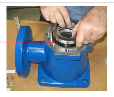
**Step 65:** Place 2 washers into counterbores. Place anti-seize on 2 bolts and inset into tapped holes.
