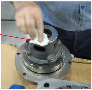
**Step 69:** Carefully insert Rotor Assembly into front of Housing. Align holes in Flange with holes in Gasket.
