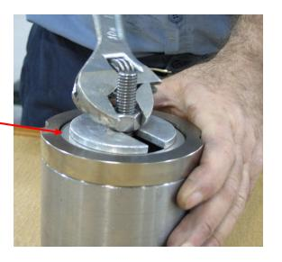
**Step 61:** Insert Retaining Ring into groove in Retaining Flange. Verify visually that Retaining Ring is fully seated.
