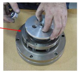
**Step 37:** Tighten down 2 screws until sleeve on screw bottoms on Flange and Carrier.
