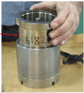
**Step 57:** Grease O-ring and insert into groove on inner diameter of Retaining Flange.
